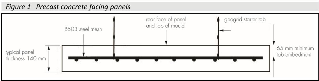
1.6 The connection detail assessed by the BBA for connection of the geogrids to the precast concrete facing panels is shown in Figure 2. A starter tab of two ribs and three transverse bars of Tensar RE500 geogrid is cast into the rear of the panel at 65 mm depth. A 100% connection efficiency can be achieved (see section 7.2).
